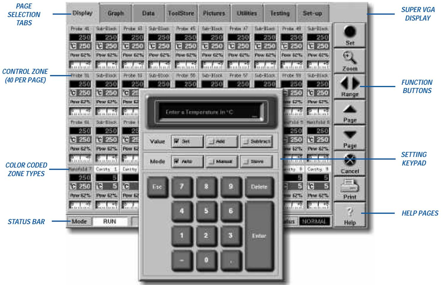
“Operator friendliness” moves to a higher level with the Athena Series HRC-TS touchscreen control console. Easy to follow visual prompts and 3-D selection buttons that move as you “press” them make setup and operation simple and virtually foolproof. Designed for maximum flexibility, the console comes network-ready, enabling remote operation.
