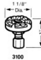
3100 Molded single or dual circuit open terminal (400°F max.). 0.2 lbs
