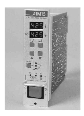
The Athena Series AIM controller features easy startup in one of three predetermined control modes selected by the user.
