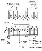
Figure 2: Typical 120 Vac for -B & -T Output
