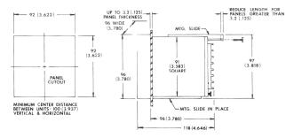
AL DIMENSIONS ARE IN MILLIMETERS; ALL DIMENSIONS ARE IN MILLIMETERS; INCHES ARE SHOWN IN PARENTHESIS. Figure 1: Cutout and case dimensions
