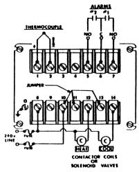
NOTE: BO and BB relay outputs rated 7 Amp @ 120V and 5 Amp @ 240V, for resistive loads only.
