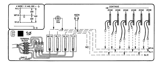
The 240 volt single-phase connection only uses two power lines plus ground.
