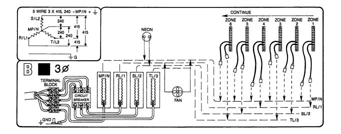
**CAUTION NOTE:** The voltages from line to line in this system are 380 to 415 volts. Severe damage to module and mainframe could result if this type of AC input system is connected in the 208-240 Vac configuration. This type of power distribution is very uncommon in the United States, but is the most common system used in other countries.
