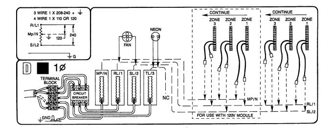
The above diagram depicts two different wiring configurations. One is 208-240 volt, single-phase, 3-wire. Note that lines RL/1 and SL/2 are connected through the circuit breaker to the appropriate terminal strips. All modules in this system will be connected between RL/1 and SL/2. MP/N is common with ground and is not connected through the circuit breaker.
